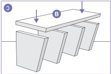
3. Now take the Seat Top (Part B) and press it firmly onto the Support Profiles making sure the sloping edge is to the front and that it overlaps the Support Profile at the front.
