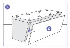
Take the Seat Front (Part C) and press it firmly over the adhesive beads on the Support Profiles.
