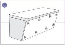
**8.** Now screw and washer fix through the seat front into each profile at the rate of two fixings per profile.
